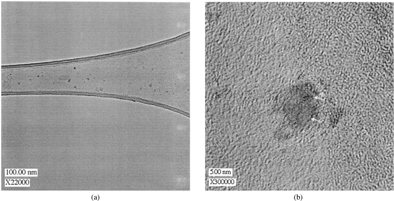
**Figure 6.** TEM micrographs of individual exhaust gas particles from a turbo-charged off-road diesel engine sampled at the location presented in Figure 1a. (a) An overview of the typical particles found on the sample presenting particles of about 40 nm in size, (b) a close-up of a typical nucleated primary particle of 5–7 nm in size.
