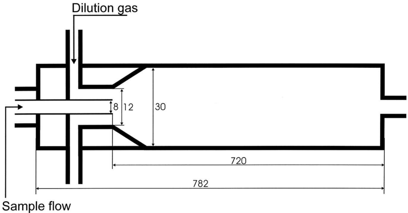
**Figure 2.** Schematics (not in scale) of the different diluters applied in this study. (a) Ejector diluter (ED), (b) partial flow diluter Smart Sampler (SS), (c) porous tube diluter (PRD). (*Continued*)
