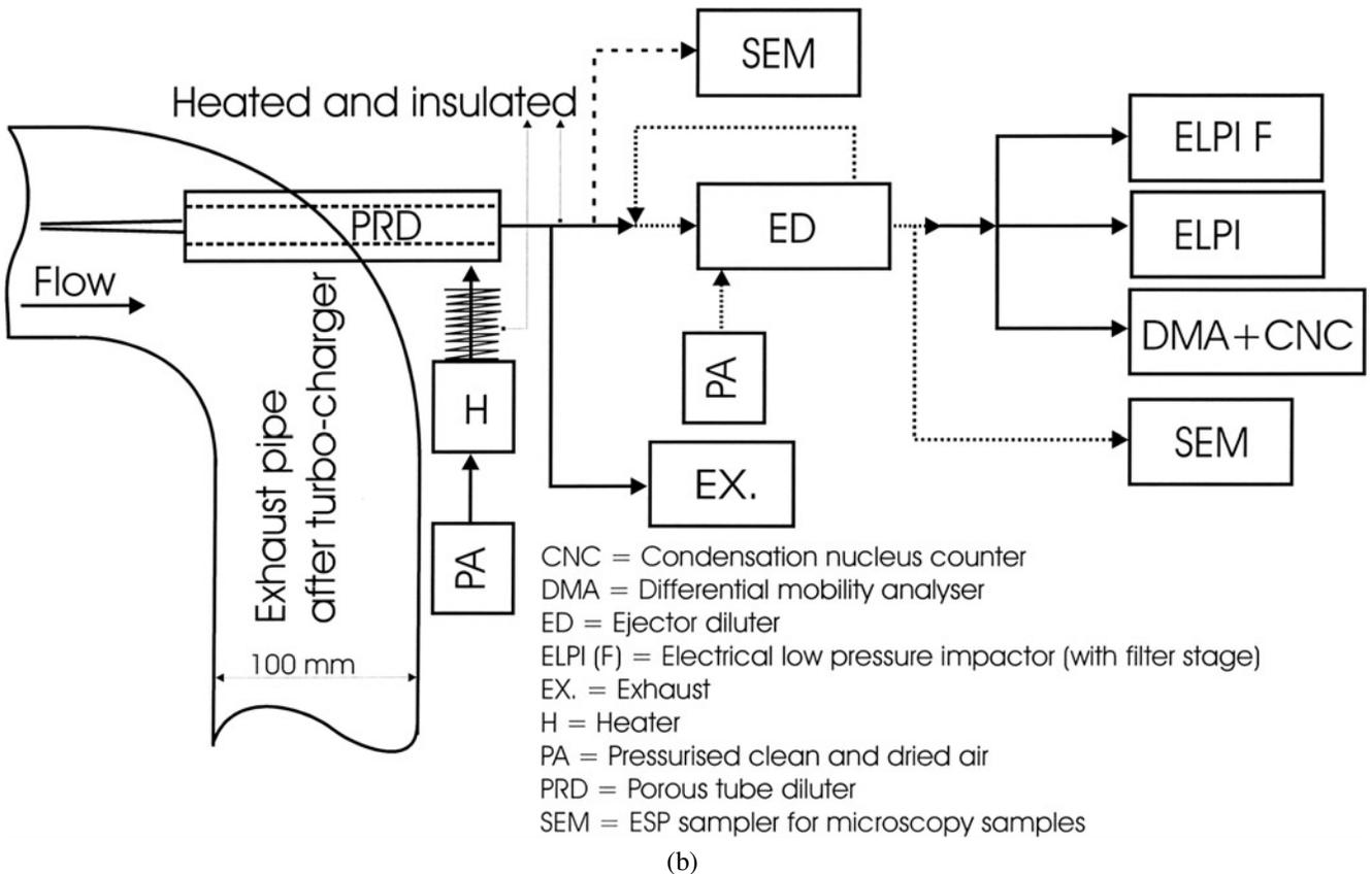
**Figure 1.** Schematics describing the different dilution setups applied in the experiments. (a) ED1 + ED2 and SS + ED, (b) PRD + ED and PRD.
