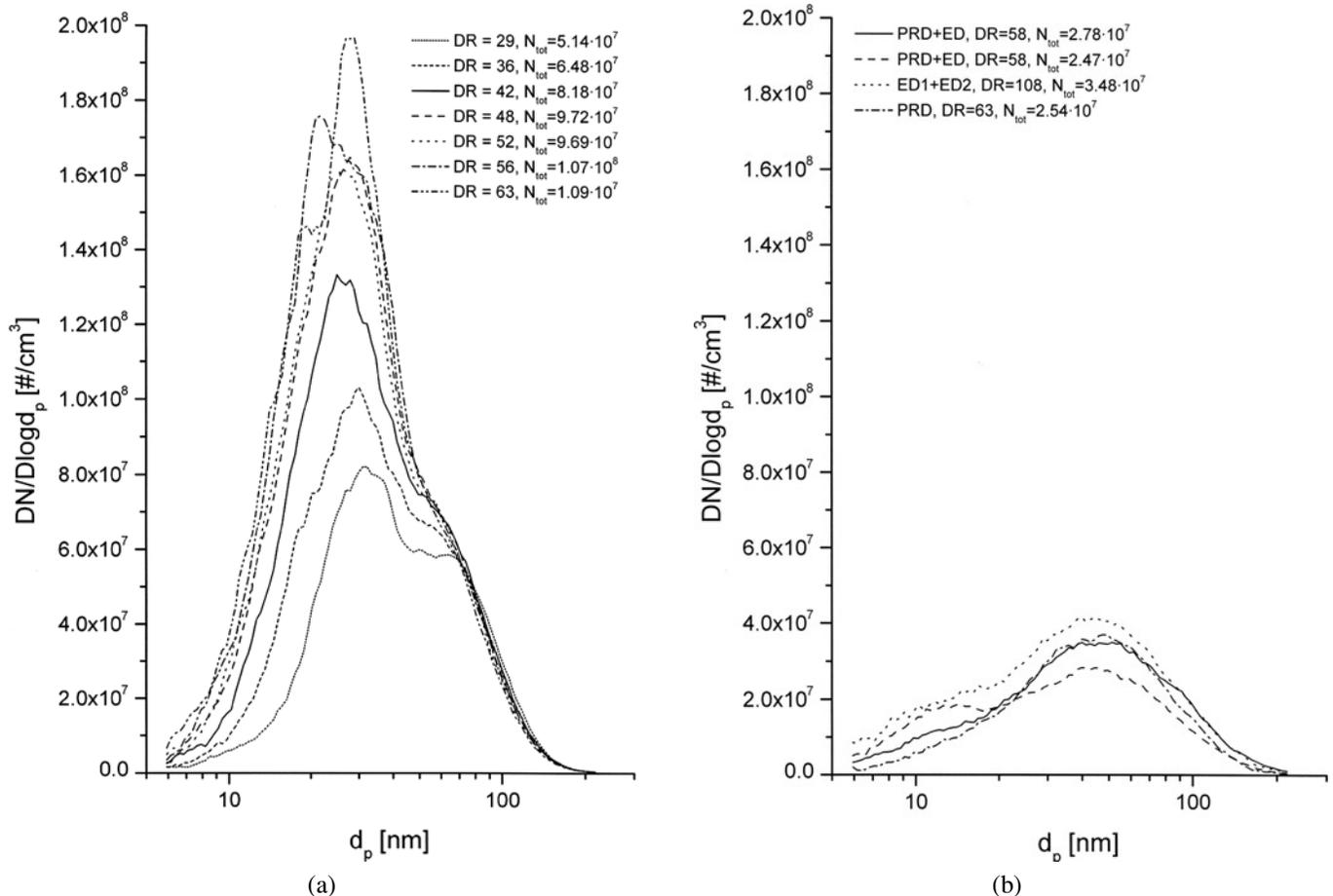
**Figure 3.** Number size distributions measured with DMA + CNC for different dilution systems and dilution ratios at low load. (a) SS + ED, (b) ED1 + ED2 and PRD + ED, (c) PRD. (Continued)
