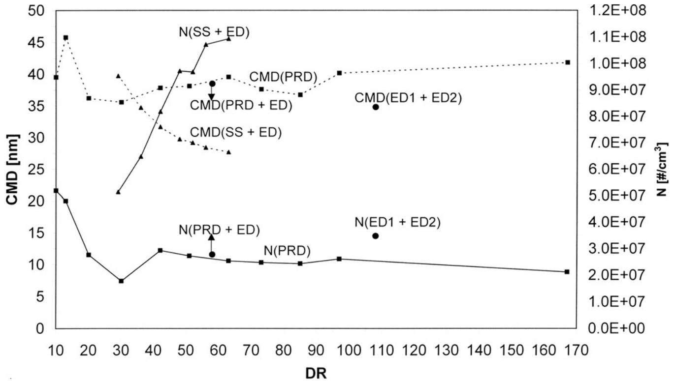
**Figure 5.** Count median diameters (CMD) together with geometric standard deviations ( $\sigma_g$ ) and total number concentrations ( $N_{tot}$ ) as a function of dilution ratio (DR) for SS + ED ( $DR(ED) = 11.7$ , constant) and PRD dilution systems.
