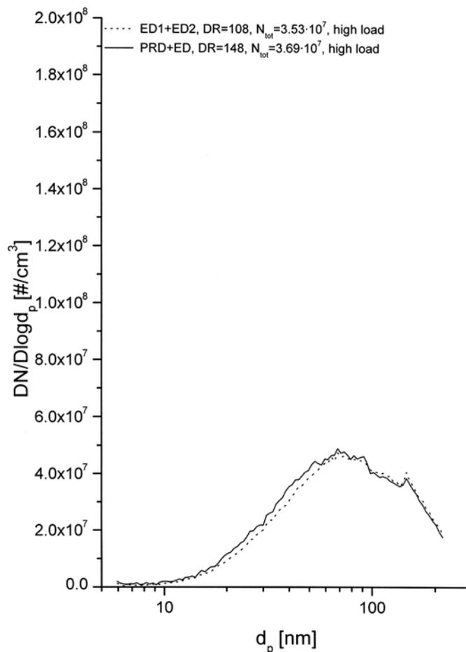
Figure 4. Number size distributions measured with DMA + CNC for different dilution systems and dilution ratios at high load.
